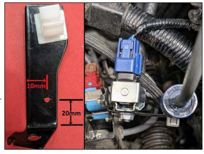
e. Connect all hoses except the 1/2" hose connected in step 8g to the supercharger as per the picture. With port 1 being closest to the throttle body the hoses connect: port 1 diff lock hose, port 2 fuel purge, port 3 brake booster and port 4 PCV.
