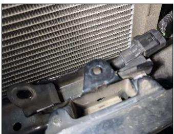
g. Fit the intercooler radiator using 3x included M6x16mm socket head cap screws and M6 flange nuts.
