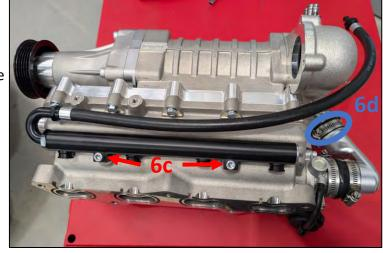
e. Undo the 12 bolts holding the upper manifold to the lower manifold noting that 2 of the bolts will be held captive in the upper manifold.
