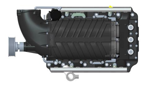
Harrop TVS2300 HEMI 5.7L with eTorque Supercharger Manifold Assembly
