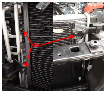
i. Secure bottom LH corner of intercooler using supplied bracket, 14562, and supplied fasteners to attach to the supercooling bottle of the air conditioning system. Use a small amount of silicone to secure bracket to bottle before tightening fasteners.
