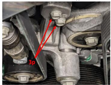
q. Remove FEAD belt from the engine. The lower tensioner has a ½" square drive underneath the pulley to fit a breaker bar with an extension.
