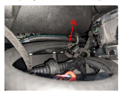
h. Using the supplied ¾" plastic hose joiner, connect the PCV vent hose (coming from the oil filler tube) to the inlet boot.
