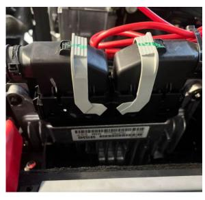
Pre 2023 RAM E-Torque – Plugs on face of ECU – Can be accessed for tuning.
