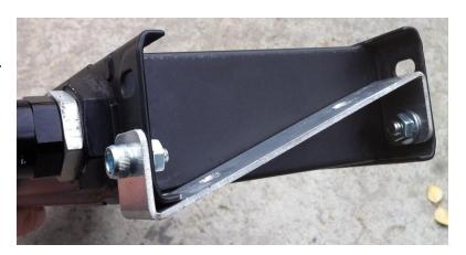
10. Assemble the M22 to dash 8 90 degree fittings to the oil cooler as shown, applying oil to the o'rings.
