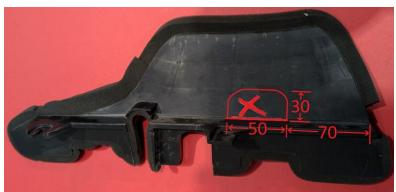
14. Drill air exit holes in lower under tray using a 60mm hole saw as per image. Ensure that the middle hole of the top row is centred on the undertray.
