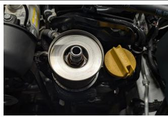
2. Assemble the dash 8 ORB to dash 8 fitting to the sandwich plate as shown. Apply lubrication to the o'ring and ensure fitting is fully seated.
