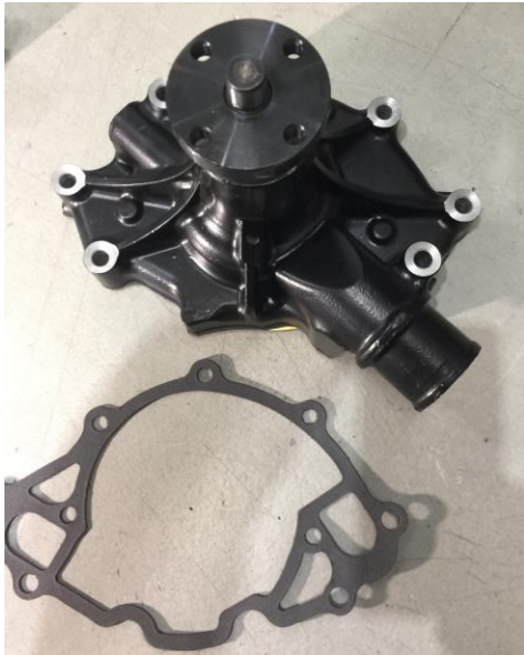
8PK Front Drive Early Style Water Pump (CVF supplied) 5.7" tall, reverse rotation, 5/8" pilot, Driver Inlet (Use with Early Model Mechanical Fuel Pump Timing Cover, or Dorman 635-100)
